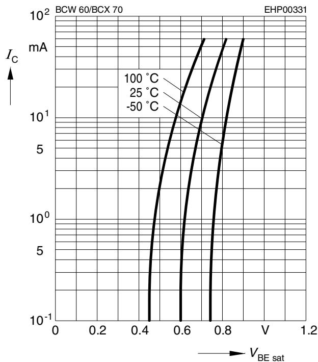
**Collector current**  $I_C = f(V_{BE})$
