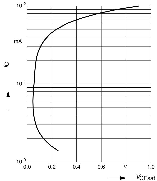
**Input off voltage**  $V_{i(off)} = f(I_C)$
