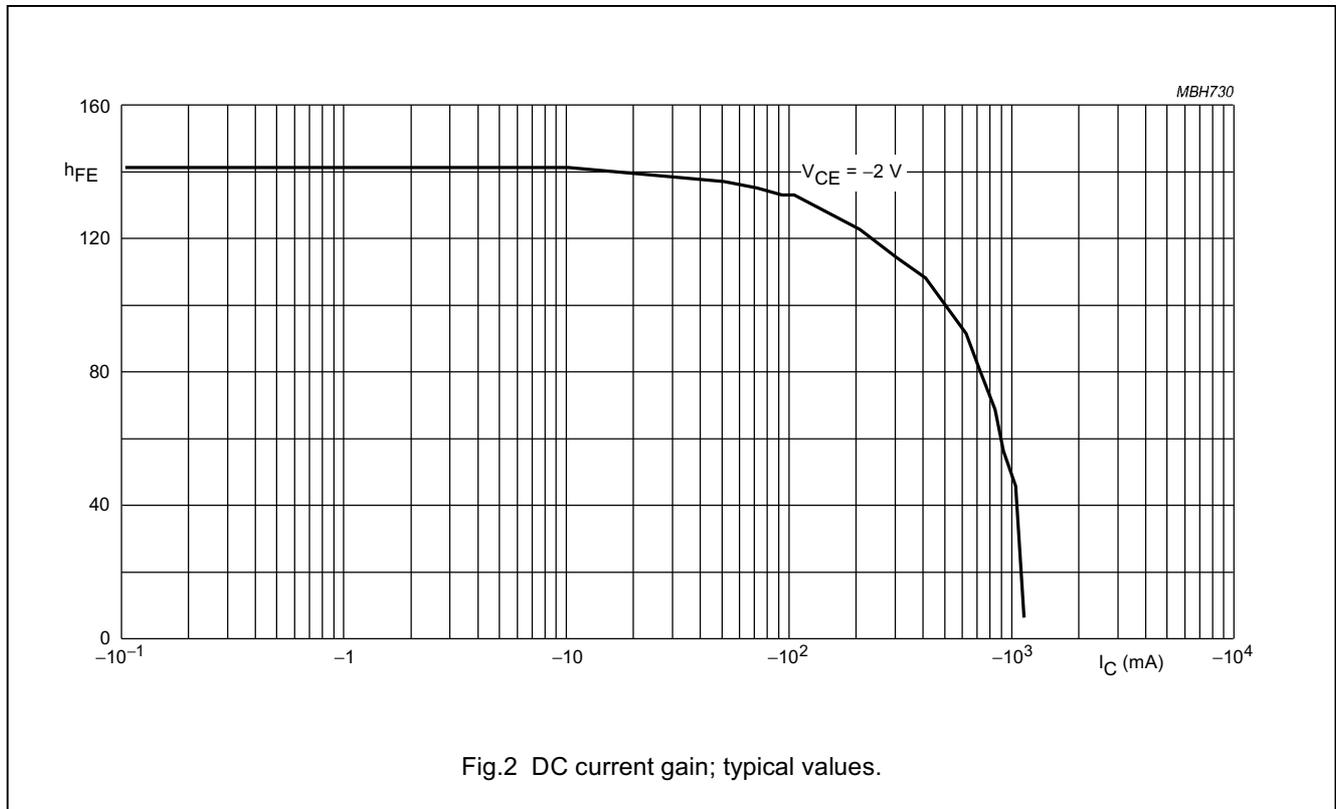
Fig.2 DC current gain; typical values.
