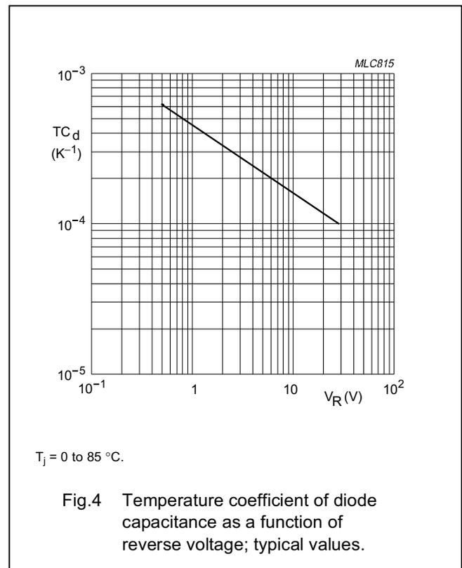
VHF variable capacitance diode
