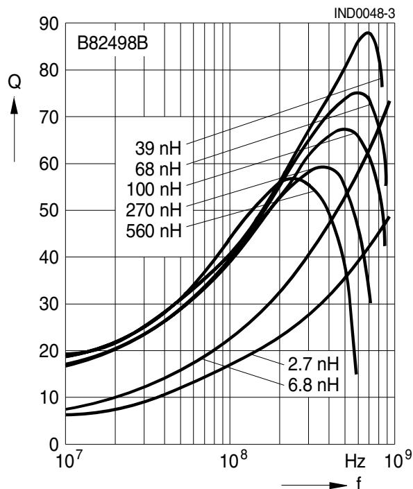
**Q factor versus frequency f (ferrite core)**
