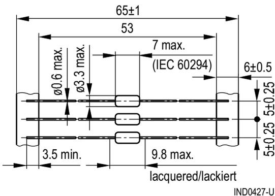
Minimum lead spacing 10 mm
