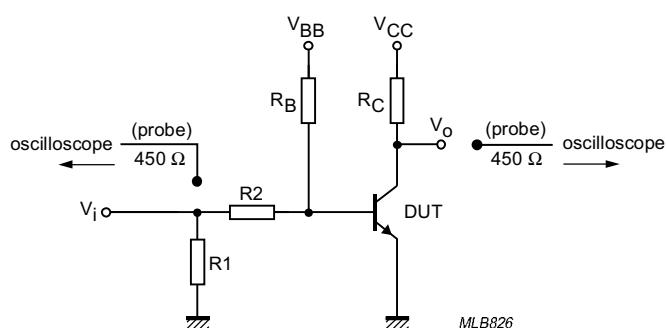
$V_i = 5$  V;  $T = 500$   $\mu$ s;  $t_p = 10$   $\mu$ s;  $t_r = t_f \leq 3$  ns.
