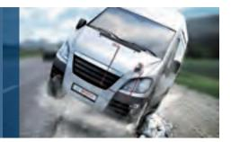
In case of an accident, a rollover situation can be securely detected with these MEMS angular rate sensors. The sensors are available with either analog or digital output. Angular rate sensors for rollover detection.
