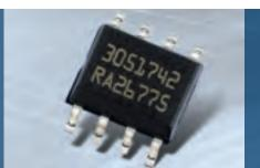
From the beginning, Bosch has been the driving force for CAN bus applications in automotive and industrial environment. A wide range of transceivers with individual features covers all applications. All devices feature a short circuit protection for the CAN bus lines.
