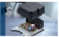
In case of an accident, MEMS acceleration sensors securely detect crash situations. They are available in various sensitivity ranges and with either analog or digital output Suitable sensor interfaces with PAS interface are described on page 7
