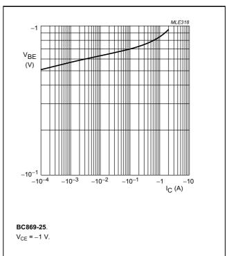
Fig.10 Base-emitter voltage as function of collector current; typical values.
