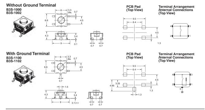
Note: Unless otherwise specified, a tolerance of ±0.4 mm applies to all dimensions. No terminal numbers are indicated on the Switches.
