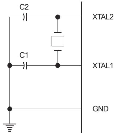
Note:  $C1, C2 = 30 \text{ pF} \pm 10 \text{ pF}$  for Crystals
