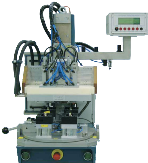
ERW thermal installation machine for embedding eight M 1.6 HITCERT® thread inserts in two mobile phone case halves
