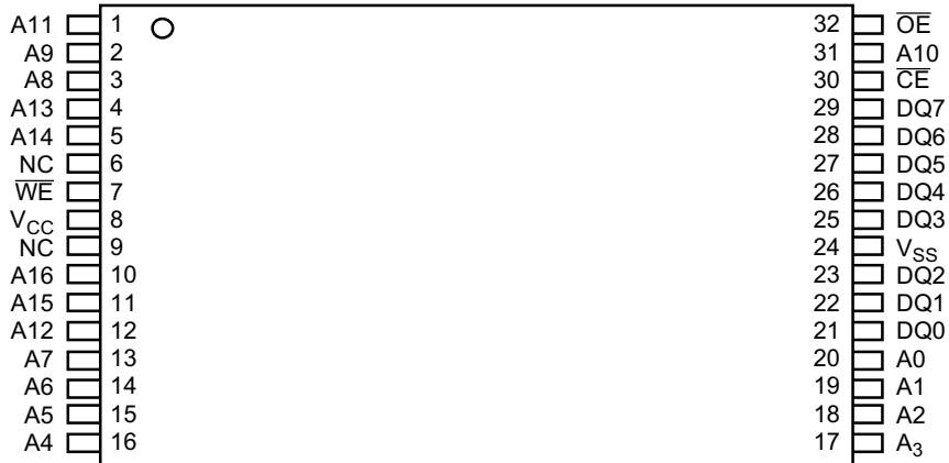
29F010 Standard Pinout
