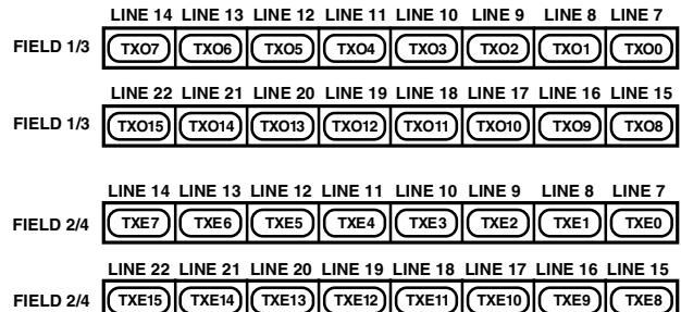
Figure 41. Teletext Control Registers
