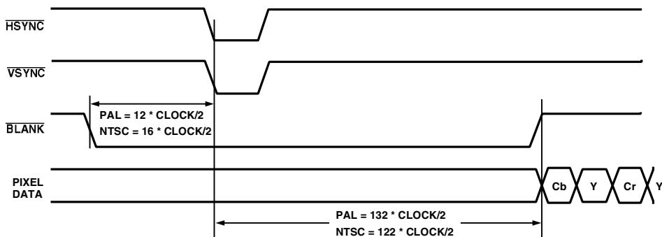
Figure 23. Timing Mode 2 Even-to-Odd Field Transition Master/Slave
