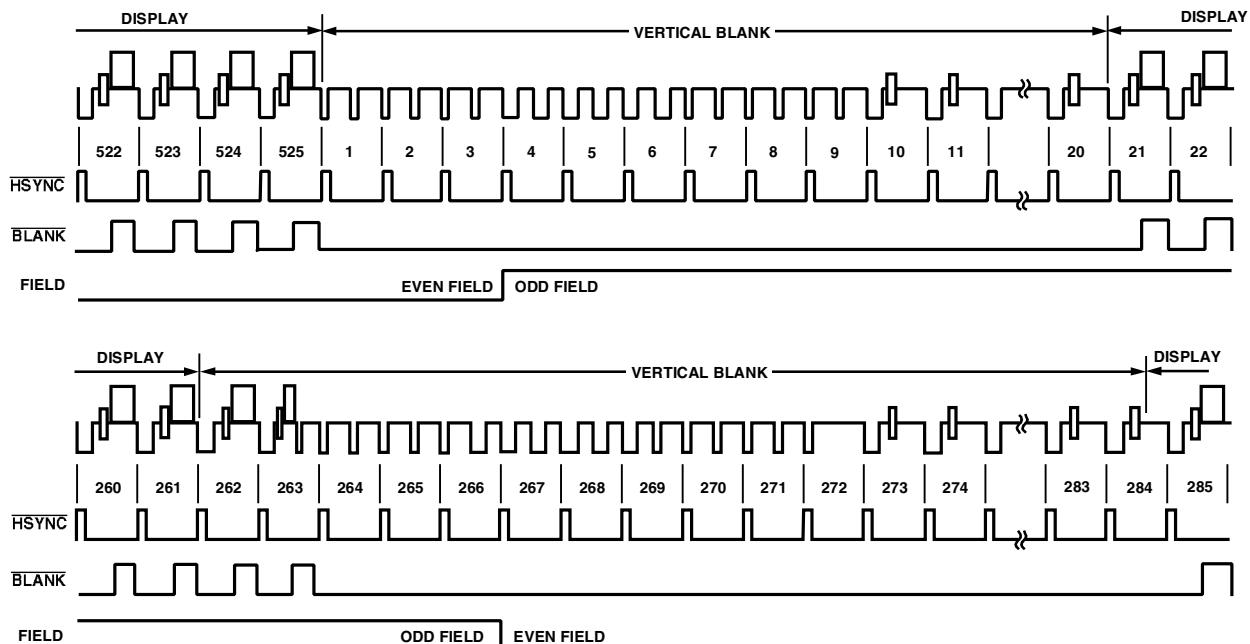
Figure 25. Timing Mode 3 (NTSC)
