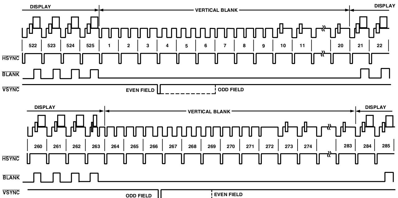
Figure 21. Timing Mode 2 (NTSC)
