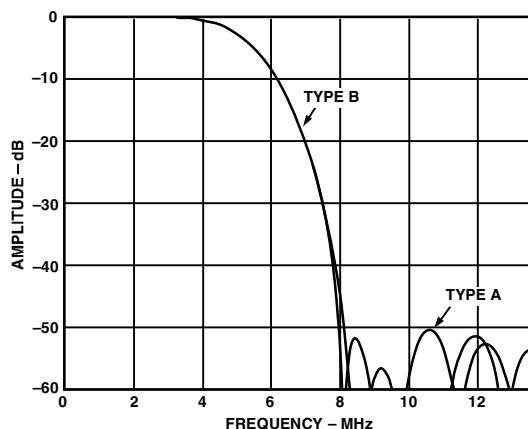
Figure 8. PAL Low-Pass Filter
