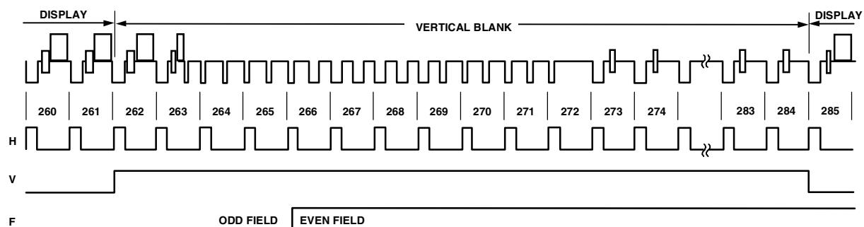
Figure 15. Timing Mode 0 (NTSC Master Mode)
