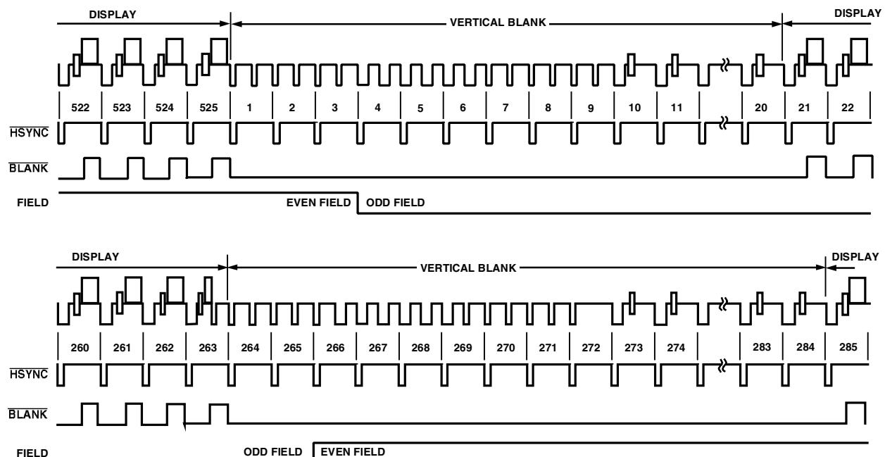
Figure 18. Timing Mode 1 (NTSC)
