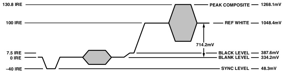
Figure 49. NTSC Composite Video Levels
