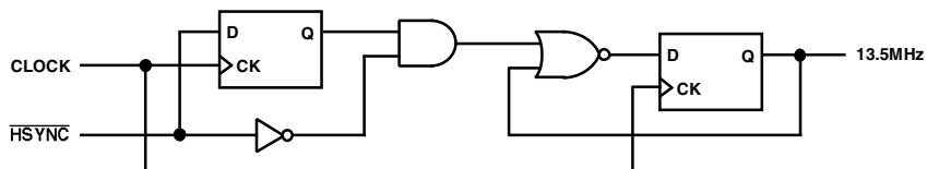
Figure 45. Circuit to Generate 13.5 MHz
