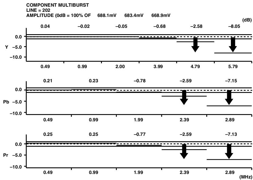
Figure 88. PAL YUV Multiburst Response
