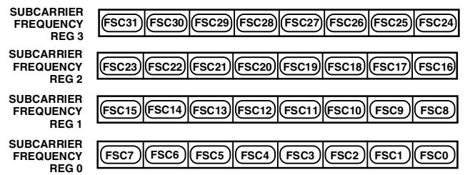
Figure 34. Subcarrier Frequency Register
