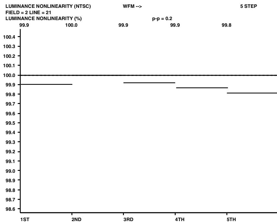
Figure 81. NTSC Luminance Nonlinearity Measurement
