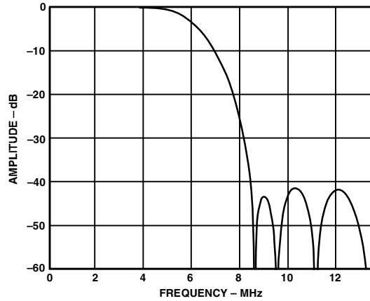
Figure 10. NTSC/PAL Extended Mode Filter
