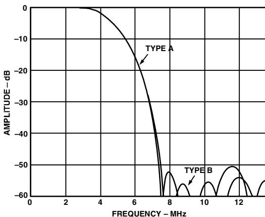
Figure 6. NTSC Low-Pass Filter
