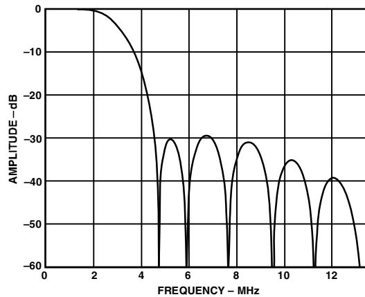
Figure 9. PAL Notch Filter
