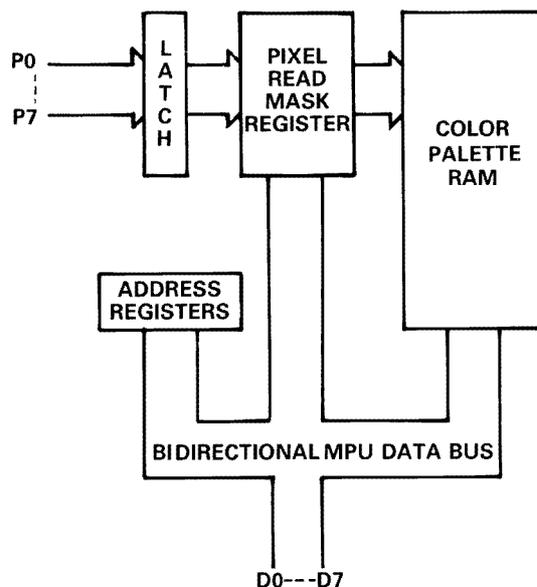
*Figure 3. Block Diagram Showing Pixel Read Mask Register*
