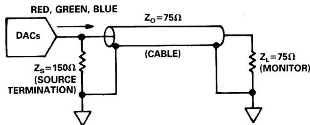
*Figure 4b. Recommended Analog Output Termination for RS-170*
