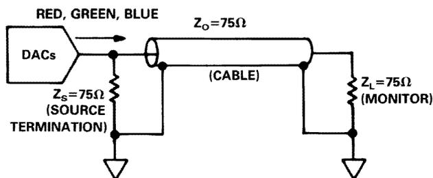
*Figure 4a. Recommended Analog Output Termination for RS-343A*
