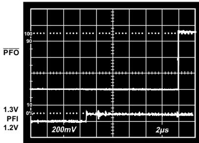
Figure 2. Power Fail Comparator Response Time L → H
