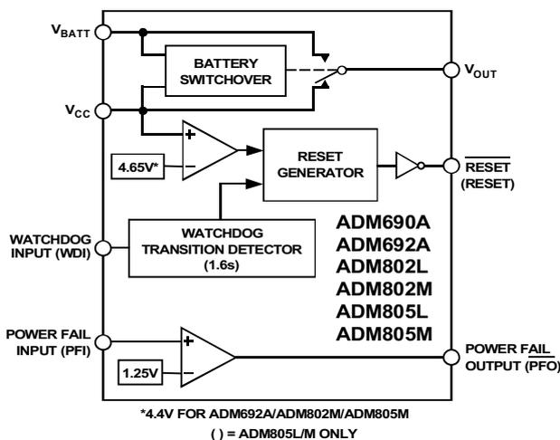
Figure 7. Functional Block Diagram
