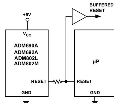
Figure 13. Bidirectional Reset
