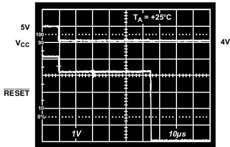
Figure 3. ADM690A  $\overline{RESET}$  Response Time
