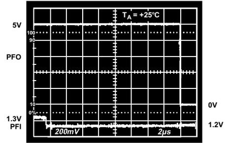
Figure 5. Power Fail Comparator Response Time H → L
