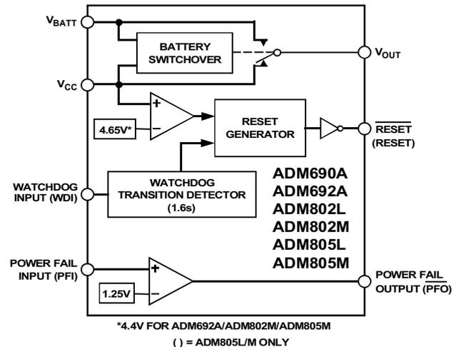
The ADM805L/M provides an active high reset output, RESET instead of  $\overline{\text{RESET}}$ .
