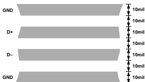
Figure 14. Arrangement of Signal Tracks
