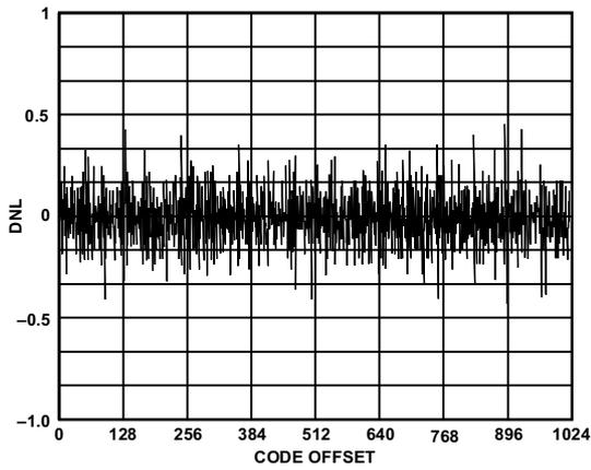
Figure 4. Typical DNL (1 V Internal Reference)
