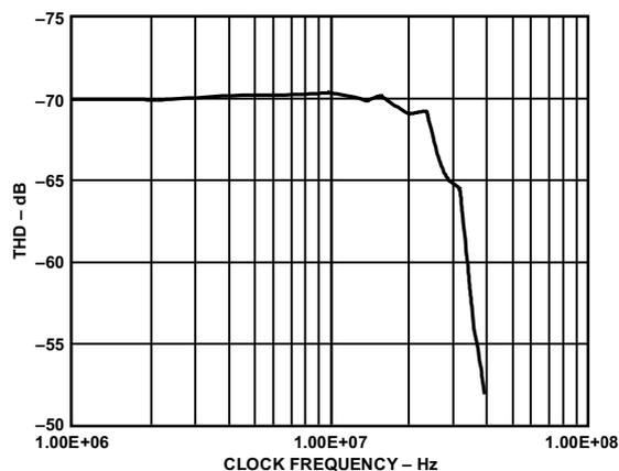
Figure 9. THD vs. Clock Frequency ( $f_{IN} = 1 \text{ MHz}$ )
