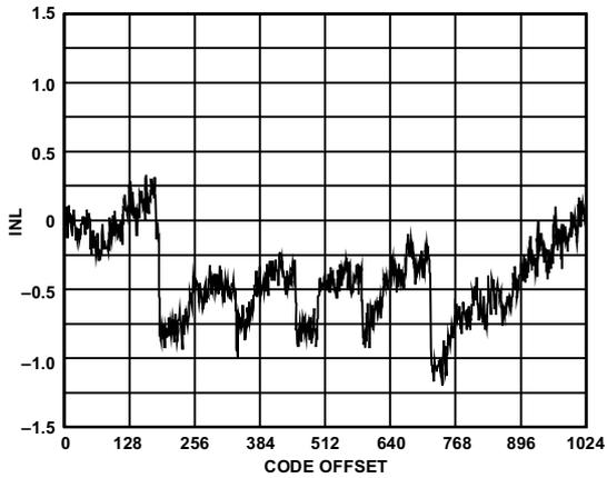
Figure 3. Typical INL (1 V Internal Reference)
