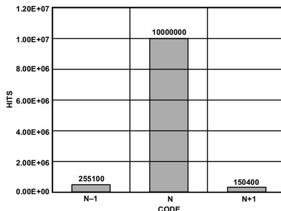
Figure 12. Grounded Input Histogram
