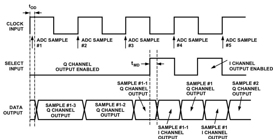
Figure 1. ADC Timing
