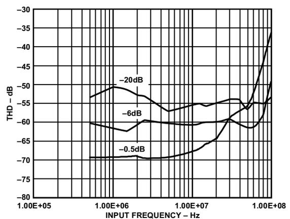
Figure 8. THD vs. Input Frequency
