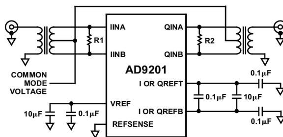
Figure 19. Example Configuration for Transformer Coupled Inputs
