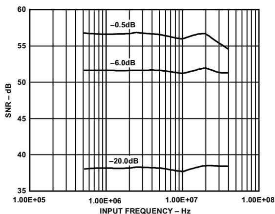
Figure 14. SNR vs. Input Frequency (Single Ended)
