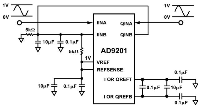
Figure 22. 0 V to 1 V Input
