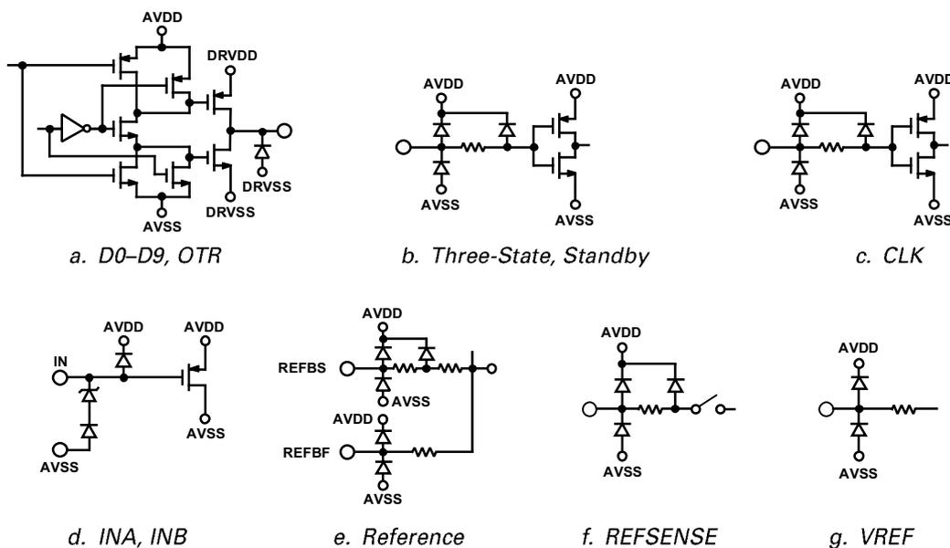
Figure 2. Equivalent Circuits
