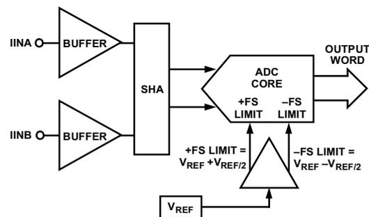
Figure 16. Equivalent Circuit for AD9201 Analog Inputs
