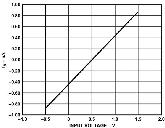
Figure 5. Input Bias Current vs. Input Voltage
