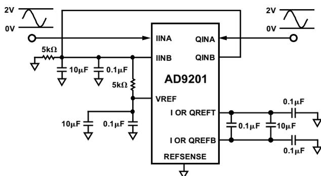
Figure 23. 0 V to 2 V Input
