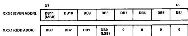
Figure 14. AD574A Data Format for 8-Bit Bus
