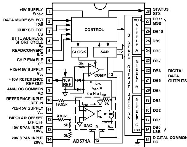
Figure 1. Block Diagram of AD574A 12-Bit A-to-D Converter
