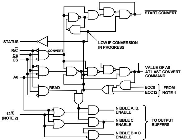
NOTE 1: WHEN START CONVERT GOES LOW, THE EOC (END OF CONVERSION) SIGNALS GO LOW. EOC8 RETURNS HIGH AFTER AN 8-BIT CONVERSION CYCLE IS COMPLETE, AND EOC12 RETURNS HIGH WHEN ALL 12-BITS HAVE BEEN CONVERTED. THE EOC SIGNALS PREVENT DATA FROM BEING READ DURING CONVERSIONS.
