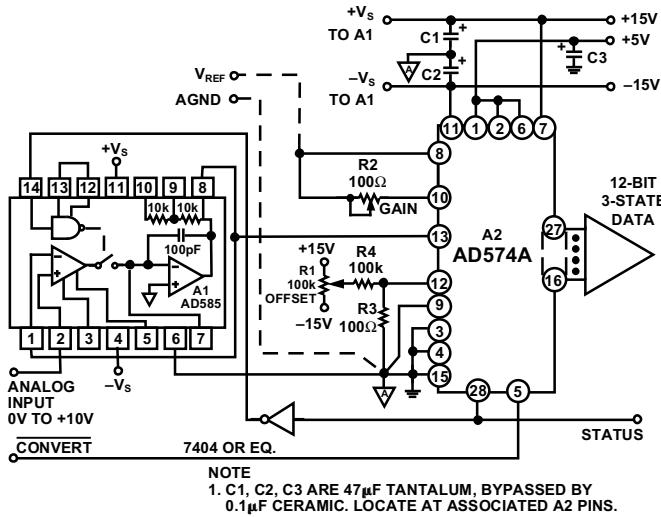
Figure 3. AD574A with AD585 Sample and Hold
