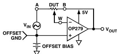
Figure 10. Inverting Gain Test Circuit
