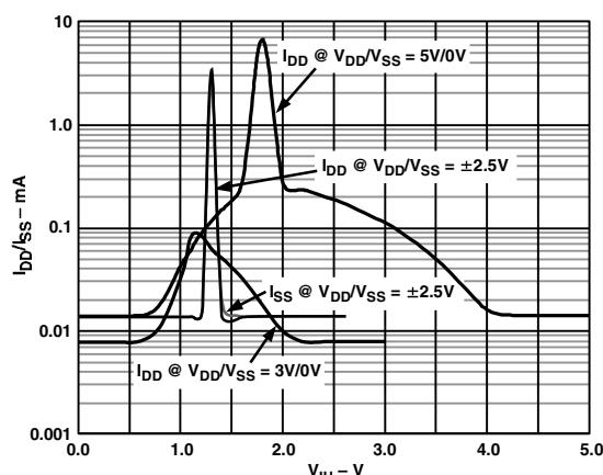
TPC 9. Supply Current vs. Logic Input Voltage
