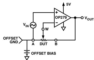
Figure 11. Noninverting Gain Test Circuit
