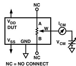
Figure 14. Common-Mode Leakage Current Test Circuit
