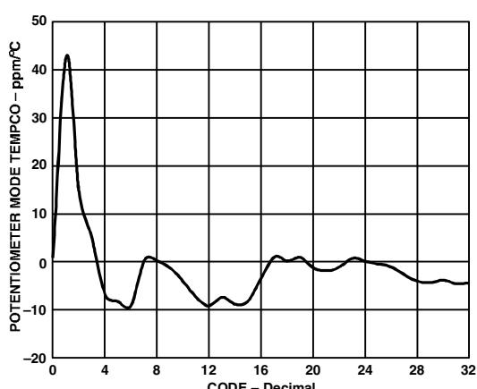
TPC 30.  $\Delta V_{WB}/\Delta T$  Potentiometer Mode Tempco
