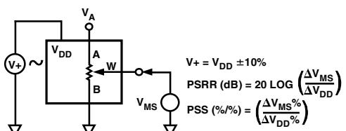
Figure 9. Power Supply Sensitivity Test Circuit (PSS, PSRR)
