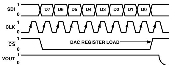
Figure 1a. AD5200 Timing Diagram
