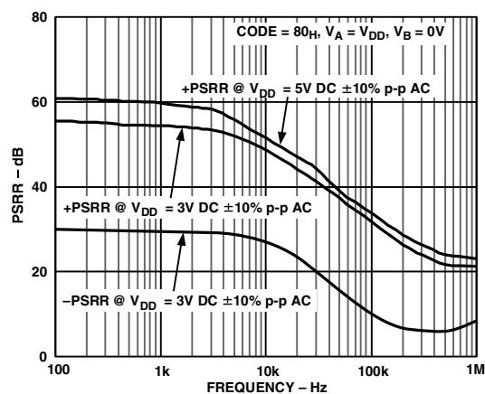
TPC 15. Power Supply Rejection Ratio vs. Frequency
