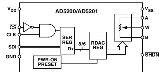
Figure 3. Block Diagram
