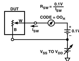
Figure 13. Incremental ON Resistance Test Circuit
