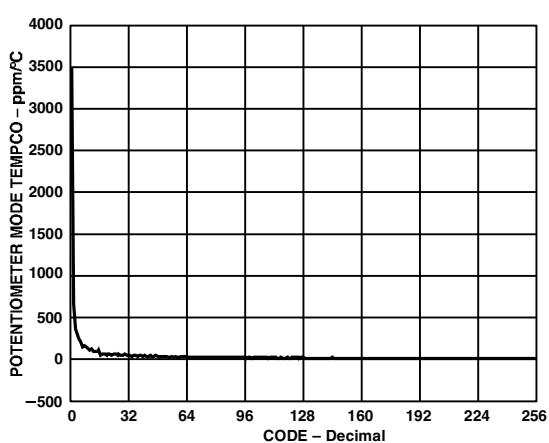
TPC 27.  $\Delta V_{WB}/\Delta T$  Potentiometer Mode Temperature Coefficient
