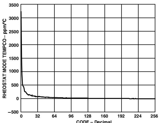
TPC 28.  $\Delta R_{WB}/\Delta T$  Rheostat Mode Temperature Coefficient
