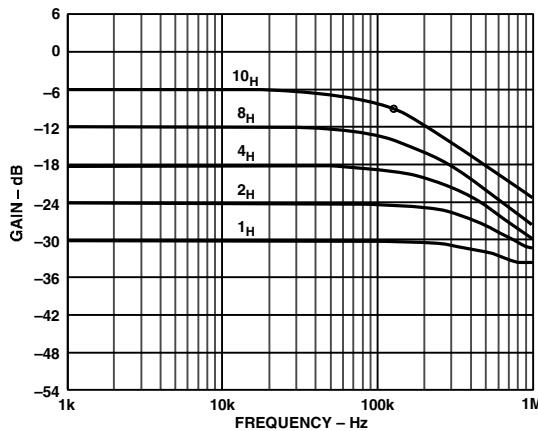
TPC 19. AD5201 50 k $\Omega$  Gain vs. Frequency vs. Code
