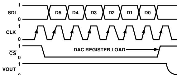
Figure 1b. AD5201 Timing Diagram
