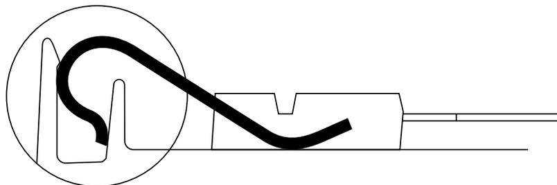
The Max Clip System comprises a proprietary reduced fin system incorporated into each heat sink into which a clip is pressed for optimum retention
