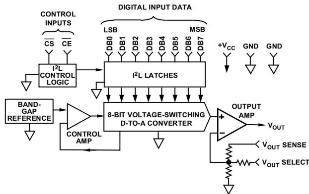
Figure 2. AD558 Functional Block Diagram
