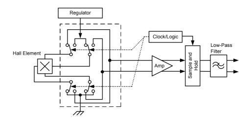
Figure 2. Model of chopper stabilization technique
