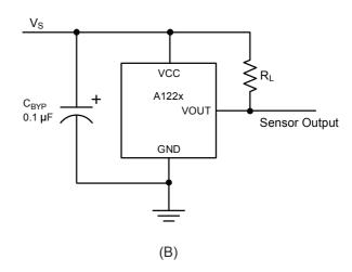
Figure 1. Switching behavior of latches. In panel A, on the horizontal axis, the B+ direction indicates increasing south polarity magnetic field strength, and the B- direction indicates decreasing south polarity field strength (including the case of increasing north polarity). This behavior can be exhibited when using a circuit such as that shown in panel B.
