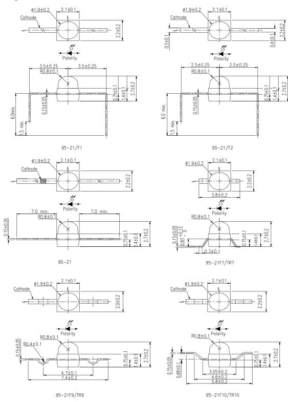
**Note:** The tolerances unless mentioned is  $\pm 0.1$ mm ,Unit = mm
