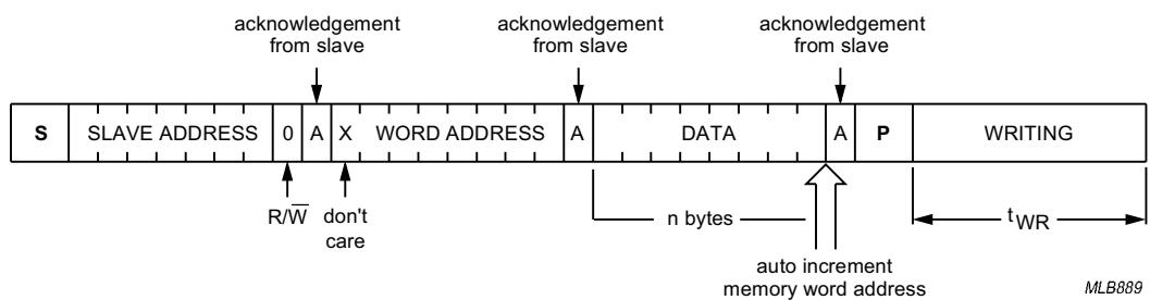
Fig.7 Master transmits to slave receiver (WRITE) mode.
