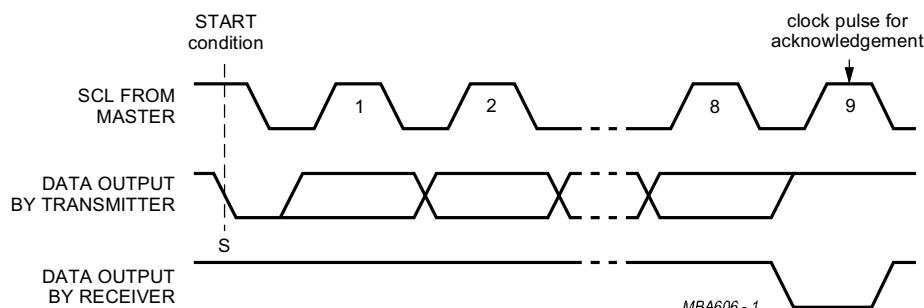
Fig.6 Acknowledgement on the I<sup>2</sup>C-bus.
