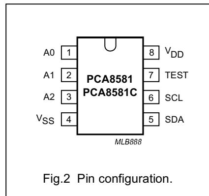
Fig.2 Pin configuration.
