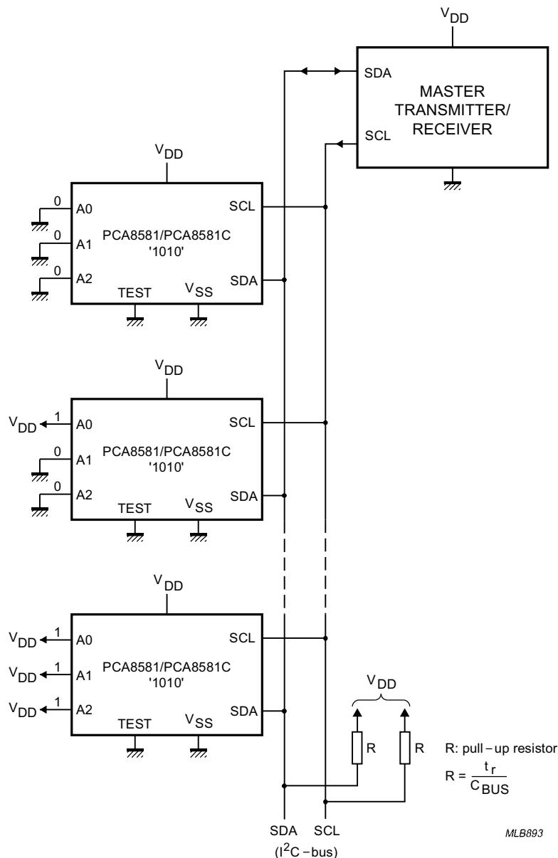
Inputs A0, A1 and A2 must be connected to V<sub>DD</sub> or V<sub>SS</sub> but not left open-circuit.
