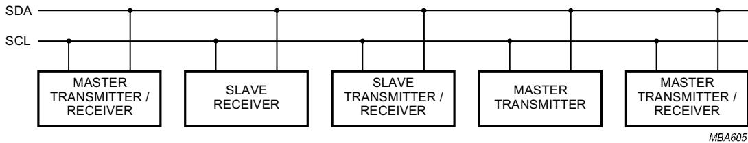
Fig.5 System configuration.
