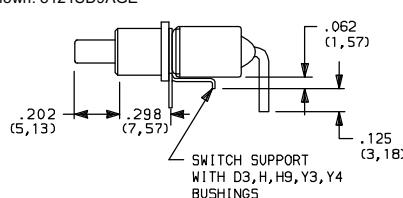
NOTE: Terminal bend radii and lead-in manufacturing option.
