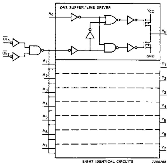
Fig.5 Logic diagram.
