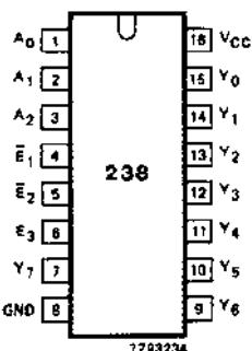
Fig.1 Pin configuration.
