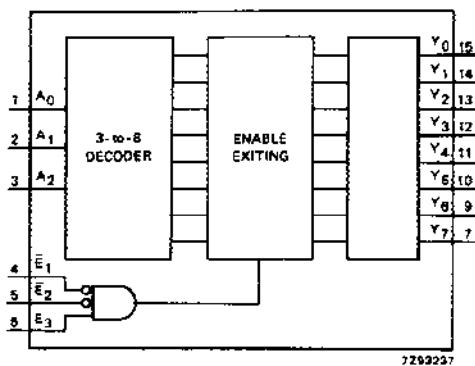
Fig.4 Functional diagram.
