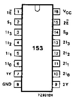
Fig.1 Pin configuration.
