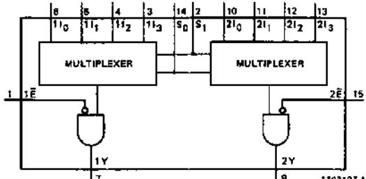
Fig.4 Functional diagram.
