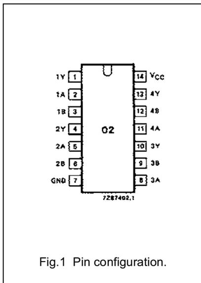
Fig.1 Pin configuration.
