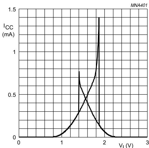
Fig.9 Typical AHC1G14 transfer characteristics;
