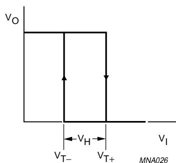
Fig.7 Transfer characteristic.
