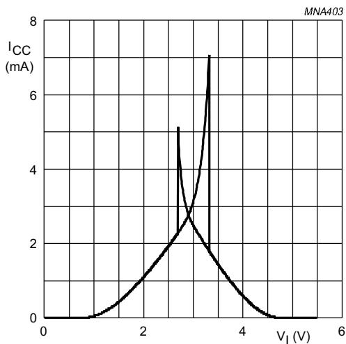
Fig.11 Typical AHC1G14 transfer characteristics;
