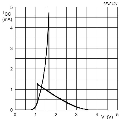
Fig.12 Typical AHCT1G14 transfer characteristics;
