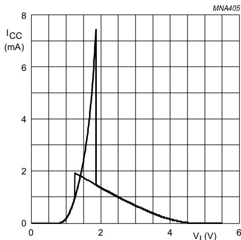
Fig.13 Typical AHCT1G14 transfer characteristics;
