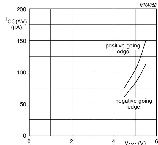
Fig.15 Average  $I_{CC}$  for AHCT1G Schmitt-trigger devices; linear change of  $V_I$  between  $0.1V_{CC}$  to  $0.9V_{CC}$ .
