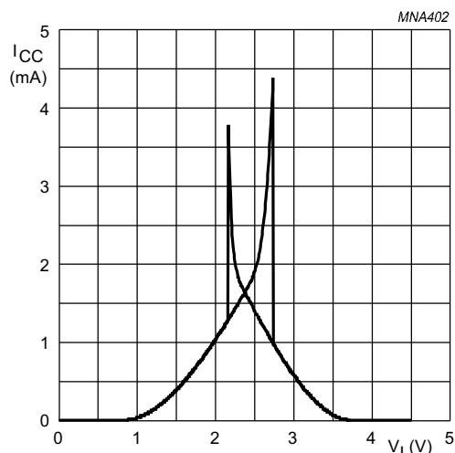
Fig.10 Typical AHC1G14 transfer characteristics;
