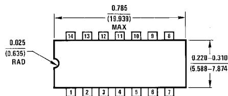
14-Lead Ceramic Dual-In-Line Package (D)
