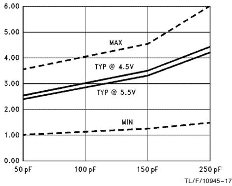
**$t_{PLH}$  vs Load Capacitance**
