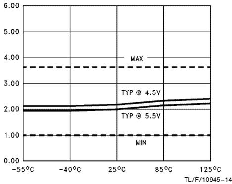
**$t_{PHL}$  vs Temperature ( $T_A$ )**
