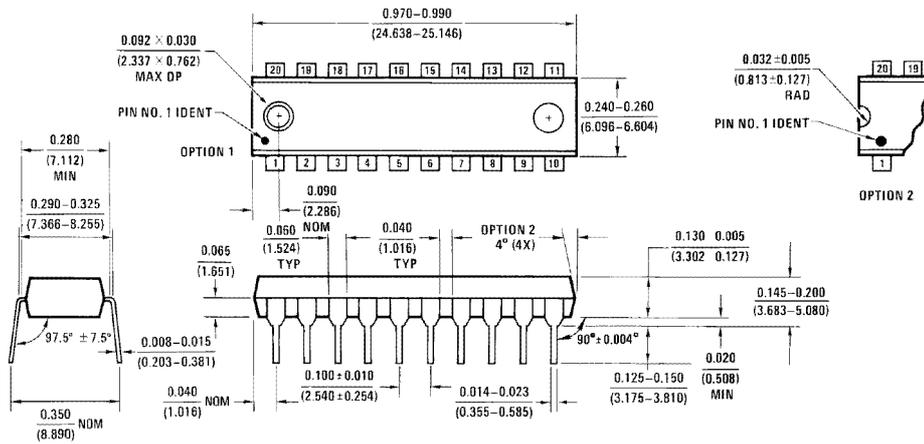
**20-Lead Plastic Dual-In-Line Package (P)
