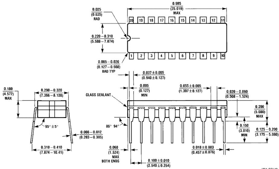
**20-Lead Ceramic Dual-In-Line Package (D)**
