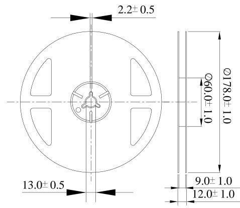
**Note** : Tolerances unless dimension ±0.1mm. Unit = mm
