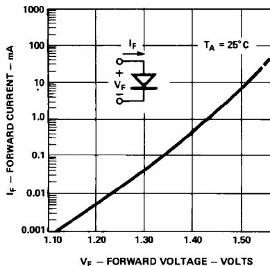
Figure 2. Input Diode Forward Current vs. Forward Voltage.
