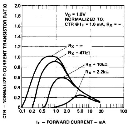
Figure 12. Effect of  $R_X$  on Current Transfer Ratio.
