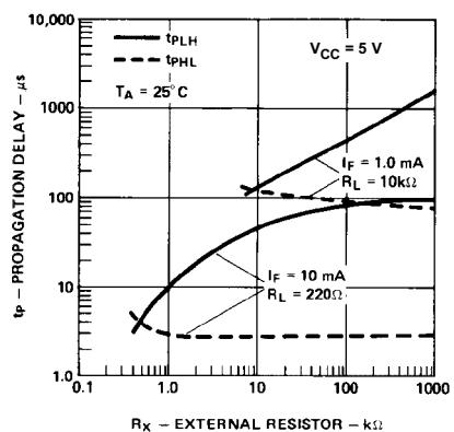
Figure 13. Effect of  $R_X$  on Propagation Delay.
