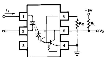
Figure 11. External Base Resistor,  $R_X$ .
