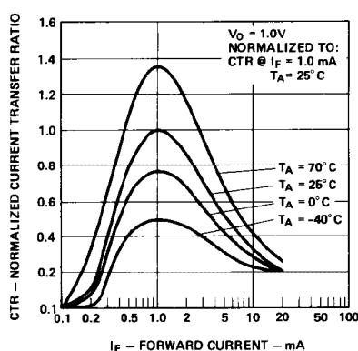
Figure 5. Current Transfer Ratio vs. Input Current.
