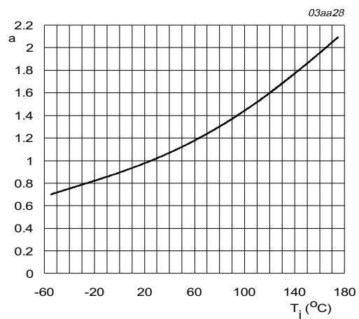
$$a = \frac{R_{DSon}}{R_{DSon}(25^\circ\text{C})}$$
