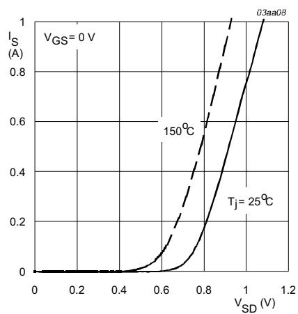
$T_j = 25^\circ\text{C}$  and  $150^\circ\text{C}$ ;  $V_{GS} = 0 \text{ V}$
