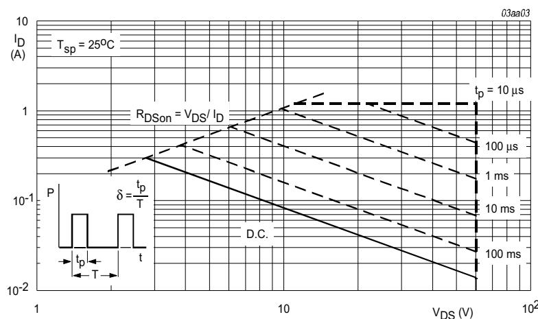
T<sub>sp</sub> = 25 °C; I<sub>DM</sub> is single pulse.
