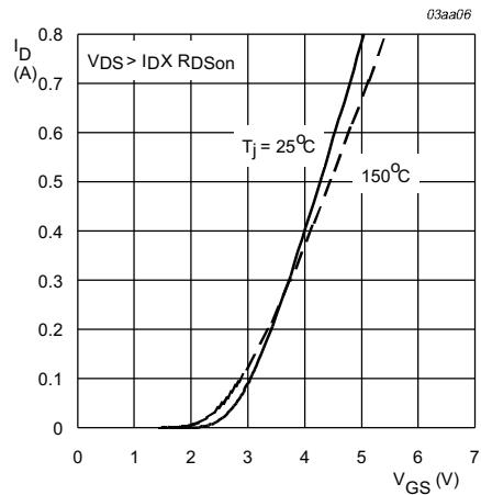
$T_j = 25^\circ\text{C}$  and  $150^\circ\text{C}$ ;  $V_{DS} > I_D \times R_{DSon}$
