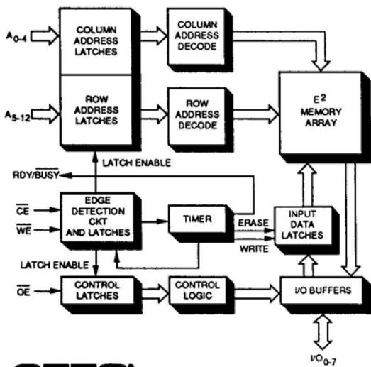
packages and has a ready/busy pin. This EEPROM is ideal for applications which require non-volatility and in-system data modification. The endurance, the number of times which a byte may be written, is a minimum of 10 thousand cycles.
