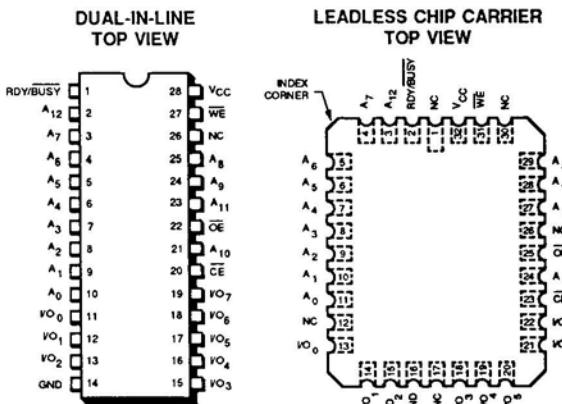
NOTE: The PLCC has the same pin configuration as the LCC except pins 1 and 17 are don't connects.
