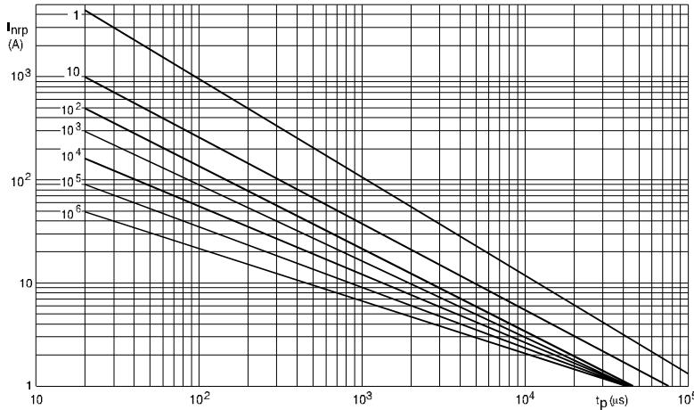
**MAXIMUM APPLICABLE TRANSIENT CURRENT AS A FUNCTION OF PULSE DURATION, 385V TO 550V (RMS); 2322 595 series.**
