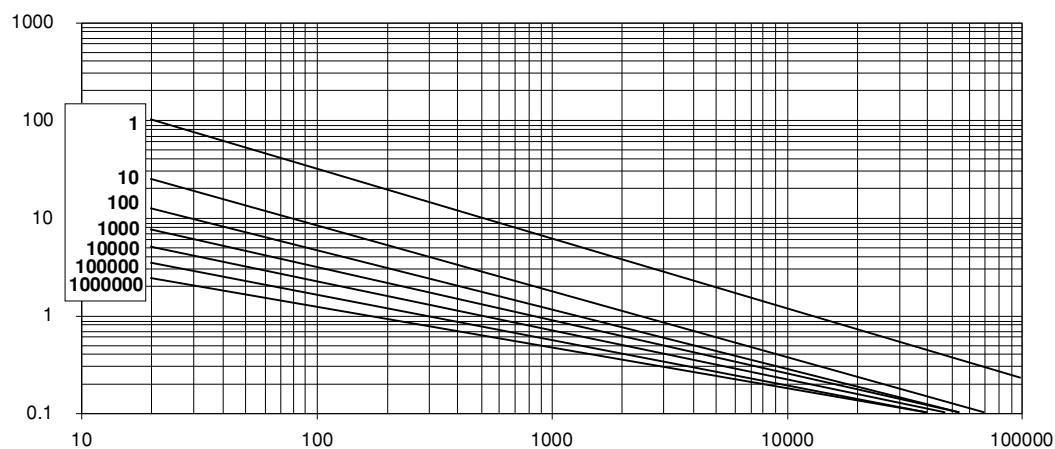
**MAXIMUM APPLICABLE TRANSIENT CURRENT AS A FUNCTION OF PULSE DURATION, 50V TO 460V (RMS); 2322 592 series.**
