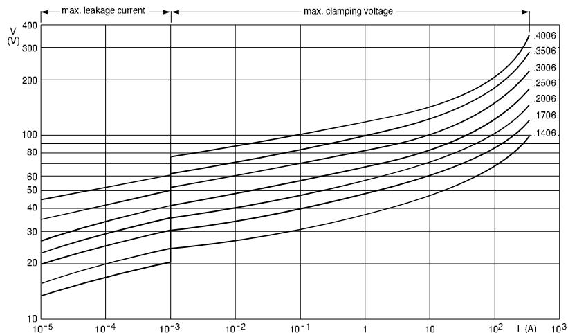
**V/I CHARACTERISTICS, 50V TO 550V (RMS); 2322 594 series.**
