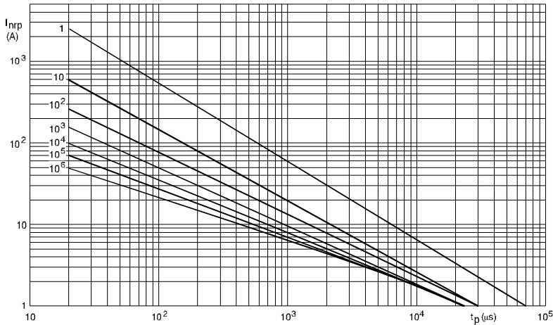
**MAXIMUM APPLICABLE TRANSIENT CURRENT AS A FUNCTION OF PULSE DURATION, 385V TO 550V (RMS); 2322 594 series.**
