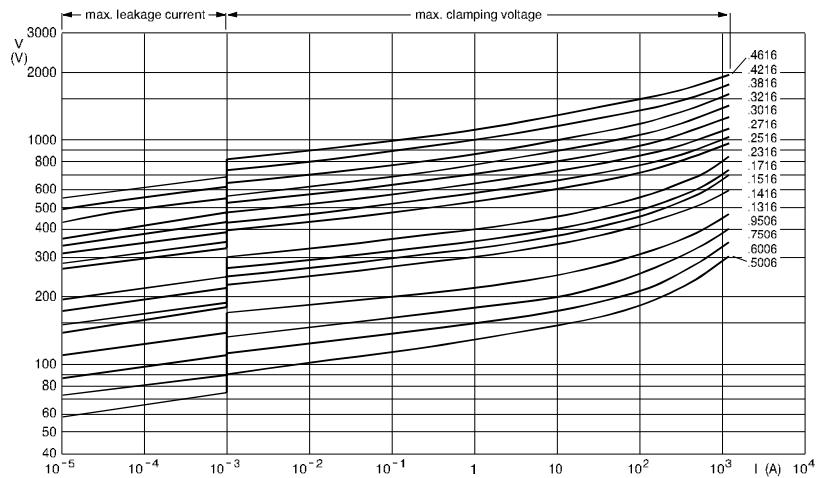
**V/I CHARACTERISTICS, 14V TO 40 V (RMS); 2322 594 series.**
