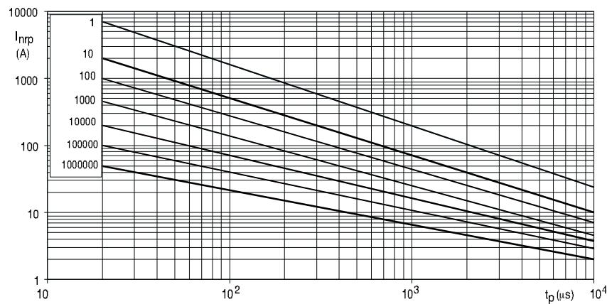
**MAXIMUM APPLICABLE TRANSIENT CURRENT AS A FUNCTION OF PULSE DURATION, 320V TO 680V (RMS); 2322 596 series.**
