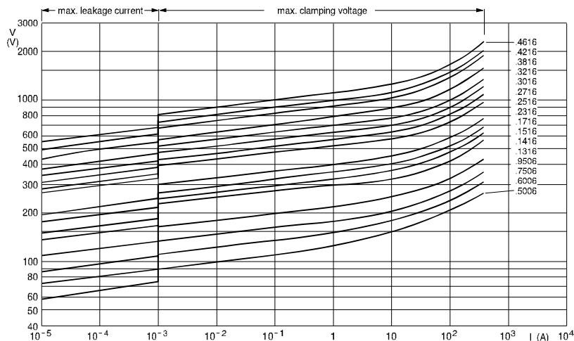
**V/I CHARACTERISTICS, 14V TO 40 V (RMS); 2322 593 series.**
