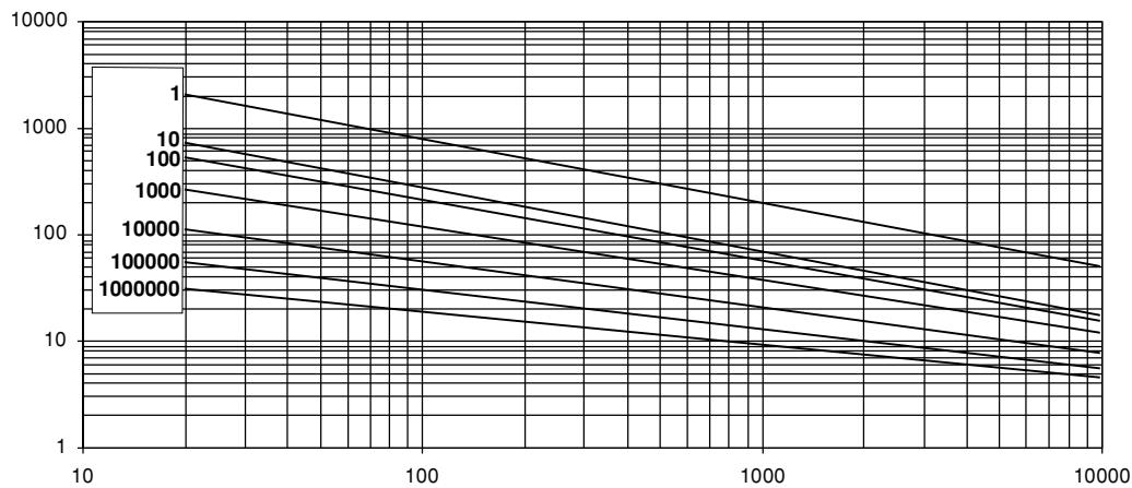
**MAXIMUM APPLICABLE TRANSIENT CURRENT AS A FUNCTION OF PULSE DURATION, 60V TO 300V (RMS); 2322 596 series.**
