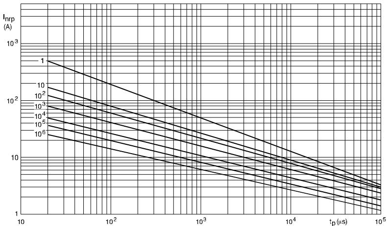
**MAXIMUM APPLICABLE TRANSIENT CURRENT AS A FUNCTION OF PULSE DURATION, 50V TO 320V (RMS); 2322 594 series.**
