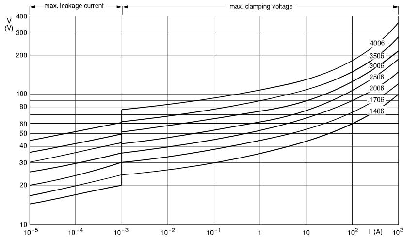
**V/I CHARACTERISTICS, 50V TO 550V (RMS); 2322 595 series.**
