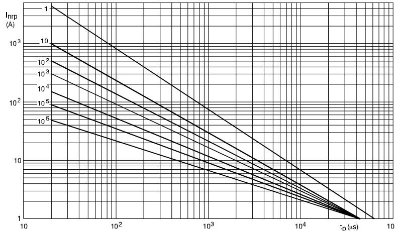
**MAXIMUM APPLICABLE TRANSIENT CURRENT AS A FUNCTION OF PULSE DURATION, 14V TO 40V (RMS); 2322 596 series.**
