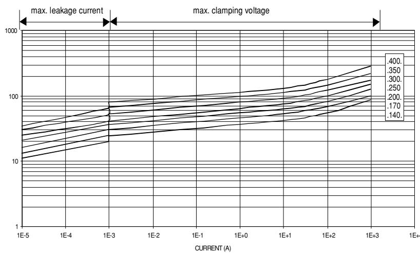
**V/I CHARACTERISTICS, 50V TO 680V (RMS); 2322 596 series.**
