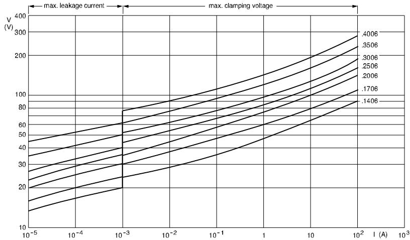
**V/I CHARACTERISTICS, 50V TO 460 V (RMS); 2322 592 series.**
