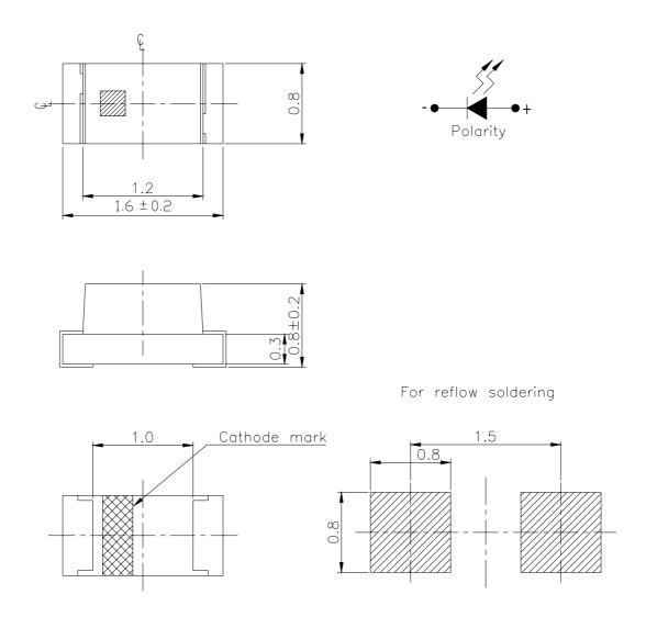
**Note:** The tolerances unless mentioned is  $\pm 0.1$ , Unit = mm
