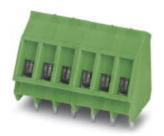
PCB terminal block, Nominal current: 24 A, Nom. voltage: 400 V, Pitch: 5 mm, Number of positions: 2, Connection method: Screw connection with tension sleeve, Mounting: Wave soldering, Conductor/PCB connection direction: 55 °, Color: green, The article can be aligned to create different nos. of positions!
