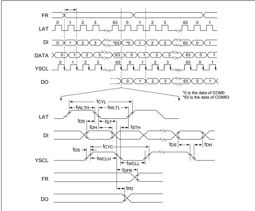
V<sub>DD</sub> = 0V, V<sub>SS</sub> = -5.0V ± 10%, T<sub>a</sub> = -20 to 75°C
