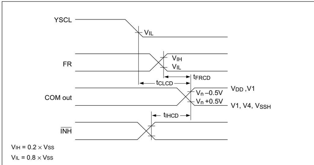
$V_{DD} = 0V, V_{SS} = -5.0V \pm 10\%, T_a = -20 \text{ to } 75^\circ\text{C}$
