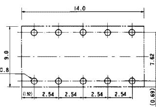
AL-D type (Double winding latching type)
