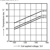
4-(2). Coil temperature rise Sample: 5 pcs., JS1a-24V Measured portion: Inside the coil Contact current: 10 A
