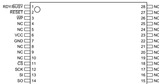
TSOP Top View Type 1
